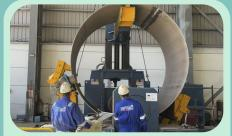
Assemblers and fabricators are responsible for fabricating and assembling wind turbine components. They use schematics, follow blueprints, conduct quality assurance, and use a variety of tools to create and align parts that meet quality standards.
